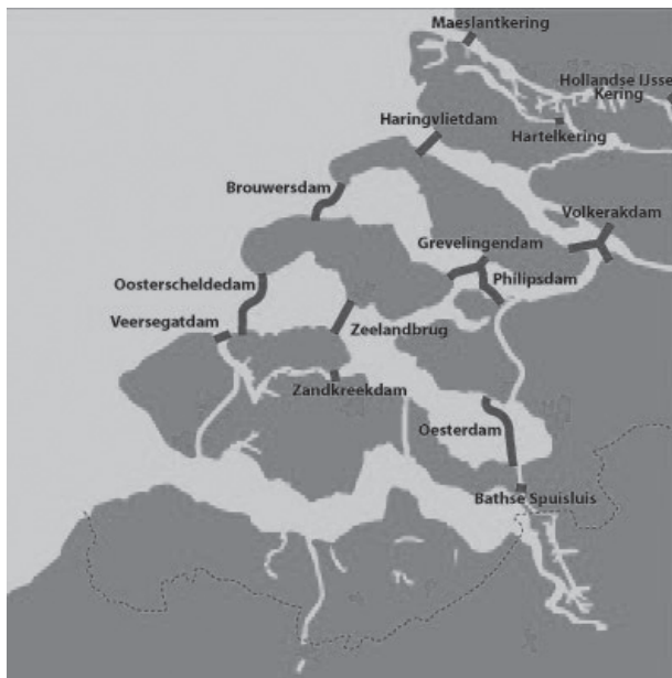
Figure 3. Locations of the storm surge barriers and dams of the Delta Plan that were constructed in the period 1958 and 1997
